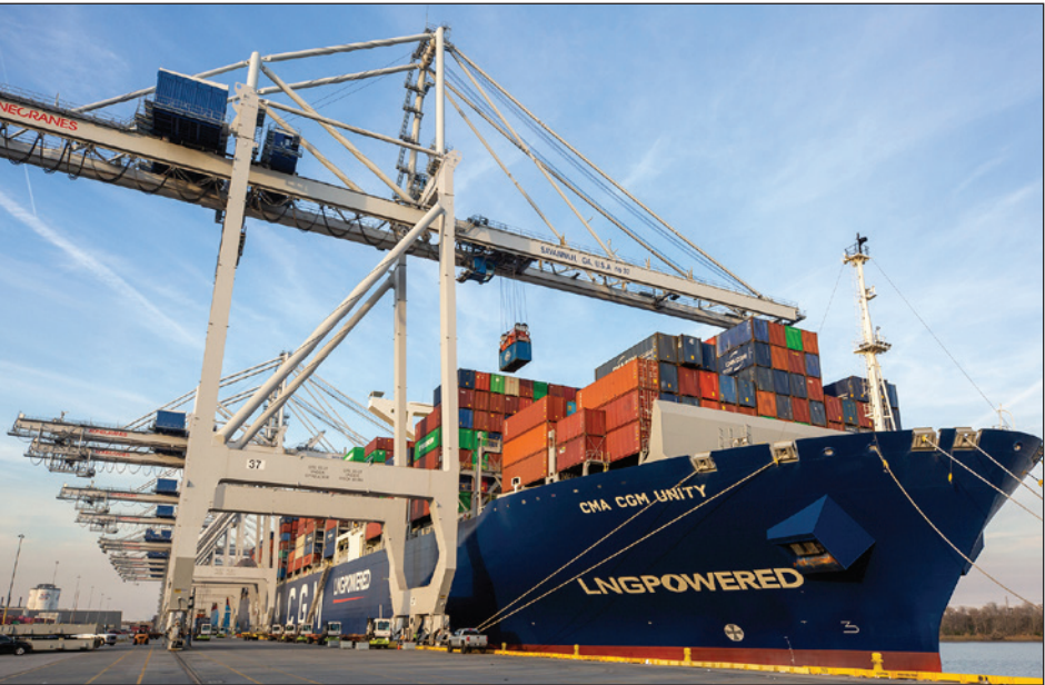
Special | Georgia Ports Authority Electric ship-to-shore cranes work the CMA CGM Unity, powered by liquefied natural gas, at the Port of Savannah’s Garden City Terminal.
